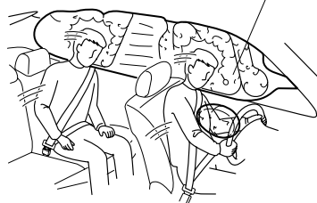
The side air bag will deploy only on the side the vehicle receives the force of the impact.
